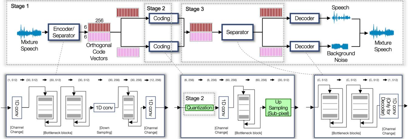
**Fig. 1:** Schematic diagram of source-aware speech coding. At Stage 1, the Stage 2 and 3 modules are not trained, while Stage 2 updates all parameters except for the Stage 3 modules. At Stage 3, all parameters are optimized.
