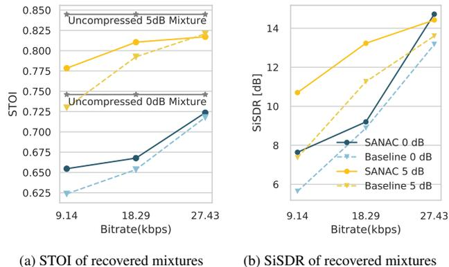
**Fig. 3:** Objective evaluation of the neural network-based models
