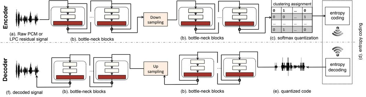
Figure 1: A schematic diagram for the end-to-end speech coding component module: some channel change steps are omitted.
